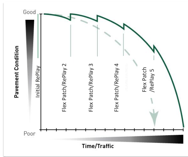
Figure 2: Typical Pavement Life Cycle with RePlay, Flex Patch & Crack Fill
